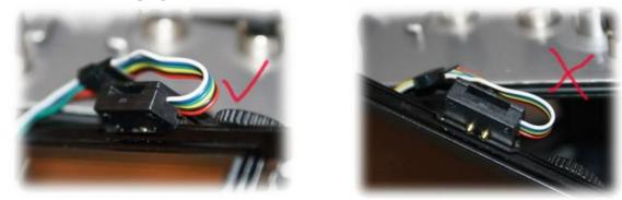
Replace the lid and make sure the lever is perpendicular to the side wall of the housing. Lock the lid by press down the lever and turn until the lever is parallel to the side wall of the housing.
